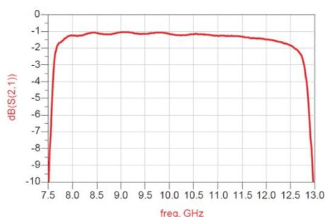
Insertion Loss & Return Loss VS Frequency (T<sub>A</sub>=25°C)
