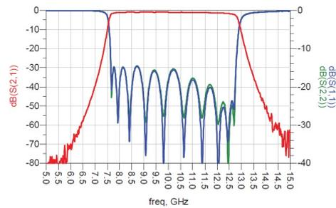
Broadband Insertion Loss VS Frequency (T<sub>A</sub>=25°C)
