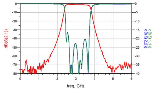
Broadband Insertion Loss VS Frequency (T<sub>A</sub>=25°C)
