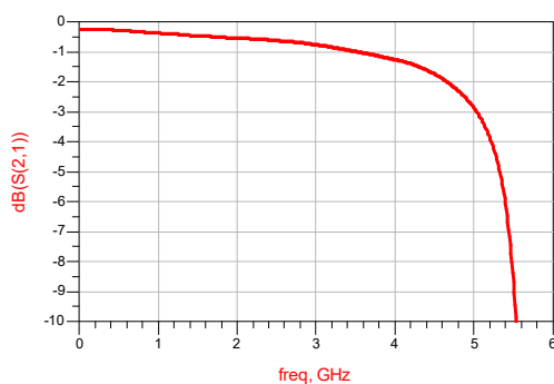
Insertion Loss VS Frequency (T A =25°C)
