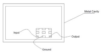
3. This filter should be soldered 2mm (at least) away from mental cavity, in order to avoid degrading filter's performance by mental cavity. Refer to the below figure.
