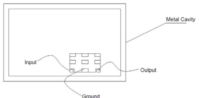
3. This filter should be soldered 2mm (at least) away from metal cavity, in order to avoid degrading filter's performance by metal cavity. Refer to the below figure.
