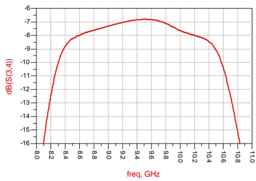
Pass band 3 Insertion Loss VS Frequency ( $T_A=25^\circ\text{C}$ )
