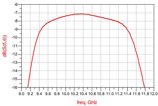
Pass band 4 Insertion Loss VS Frequency ( $T_A=25^\circ\text{C}$ )
