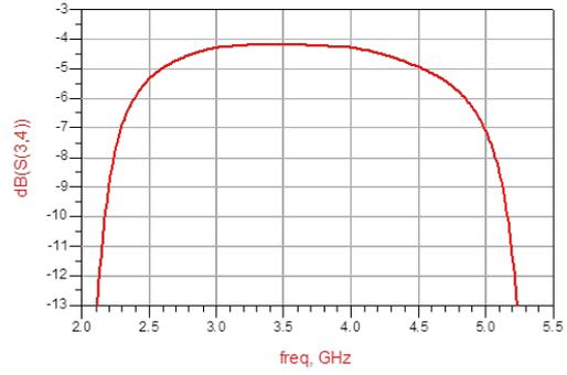
Pass band 3 Insertion Loss VS Frequency ( $T_A=25^\circ\text{C}$ )
