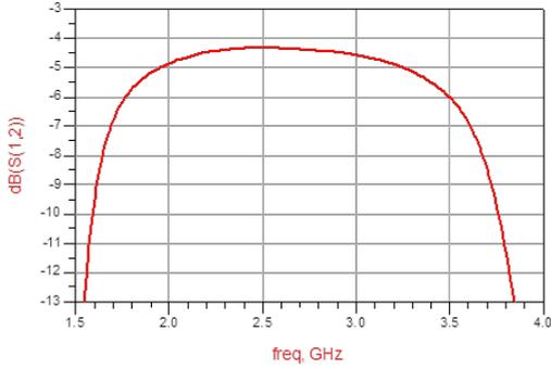
Pass band 2 Insertion Loss VS Frequency ( $T_A=25^\circ\text{C}$ )
