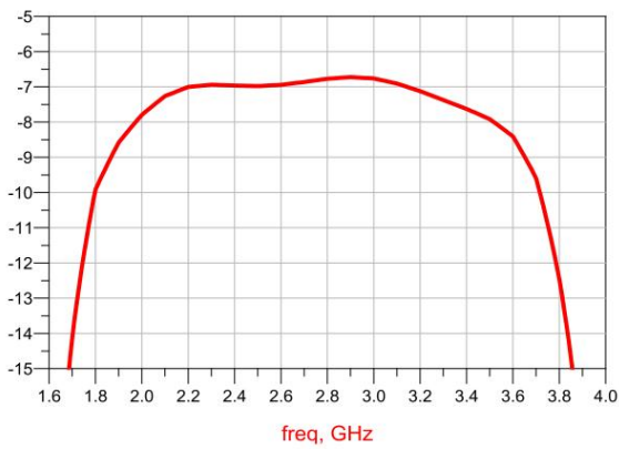
Pass band 5 Insertion Loss VS Frequency (TA=25°C)
