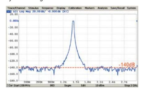
Typical dynamic range of 140 dB, typ. is achieved through the entire frequency range (10 Hz IF BW). Seen here is the maximum dynamic range achieved when using 10 IF BW and an output power level of 10 dBm.
