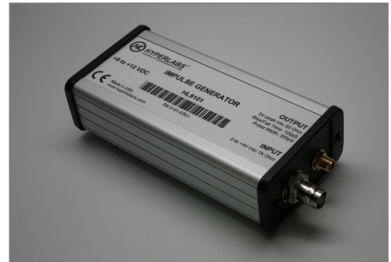
Figure 1: HL9101 Triggerable Impulse Generator (100 ps)
