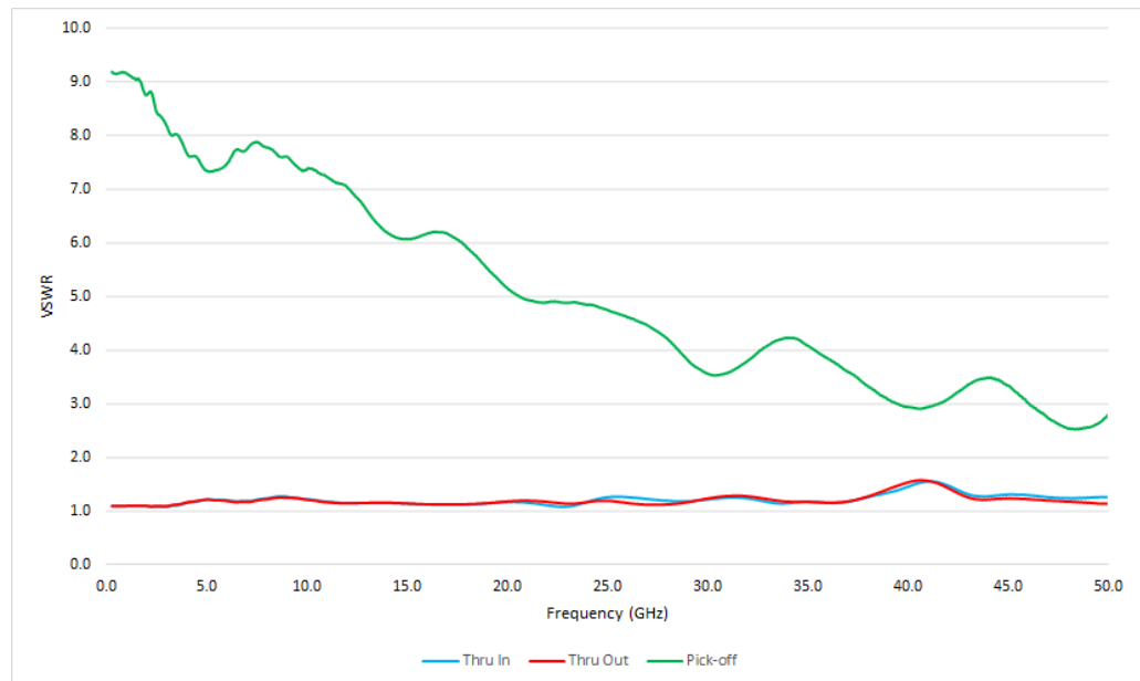
Figure 11: Typical HL9565-U-20-JJJ VSWR on all ports
